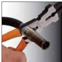
Nozzle removal & installation
