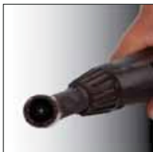
Welding Gun Nozzle filled with weld spatter
