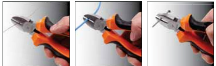
Induction hardened cutting edges (54-58 HRC) for cutting soft to medium hard wires and nails
