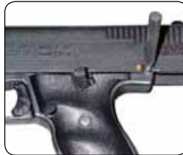
Roll Pin Punch being used to remove spring pin from a gun
