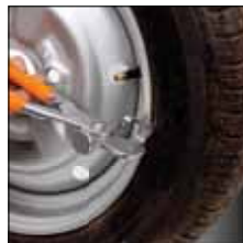
Plier being used to detach wheel balancing weights
