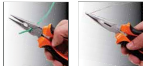
Induction hardened cutting edges (54-58 HRC) for cutting soft to medium hard wires
