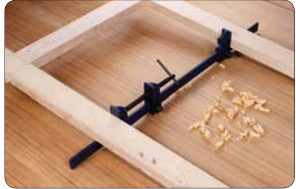
Duo Bar used for internal clamping
