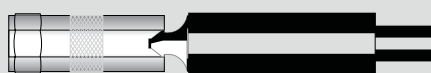
STEP 2 Snap on the system by simply "Plugging On" the grease fitting to the coupler
