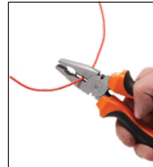
Induction hardened cutting edges (54-58 HRC) for cutting soft to medium hard wires
