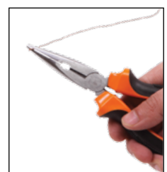
Induction hardened cutting edges (54-58 HRC) for cutting soft to medium hard wires
